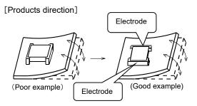
Products shall be located in the sideways direction to the mechanical stress.
