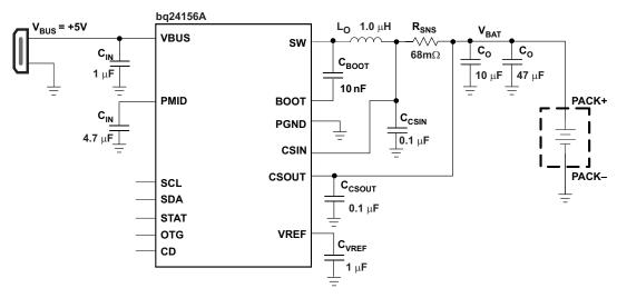
Figure 22. Battery Powered USB-DCP Power Supply
