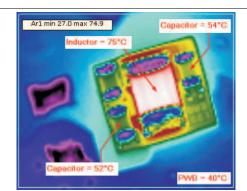
Figure 25.  $V_{IN}$ =3.6v,  $V_{OUT}$ =5v,  $I_{OUT}$ =600ma 600mw Power Dissipation At Room Temperature
