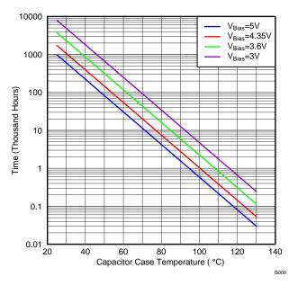
Figure 26. Capacitor Lifetime vs Capacitor Case Temperature
