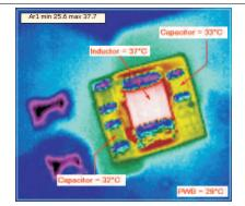
Figure 24. V<sub>IN</sub>=3.6v, V<sub>OUT</sub>=5v, I<sub>OUT</sub>=300ma 150mw Power Dissipation At Room Temperature
