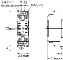
Mounting hole PYF14A series PYF14A-E PYFZ-14 serie PYFZ-14-E Screw wiring/Fixture rail/Dimensions PYF14A series
