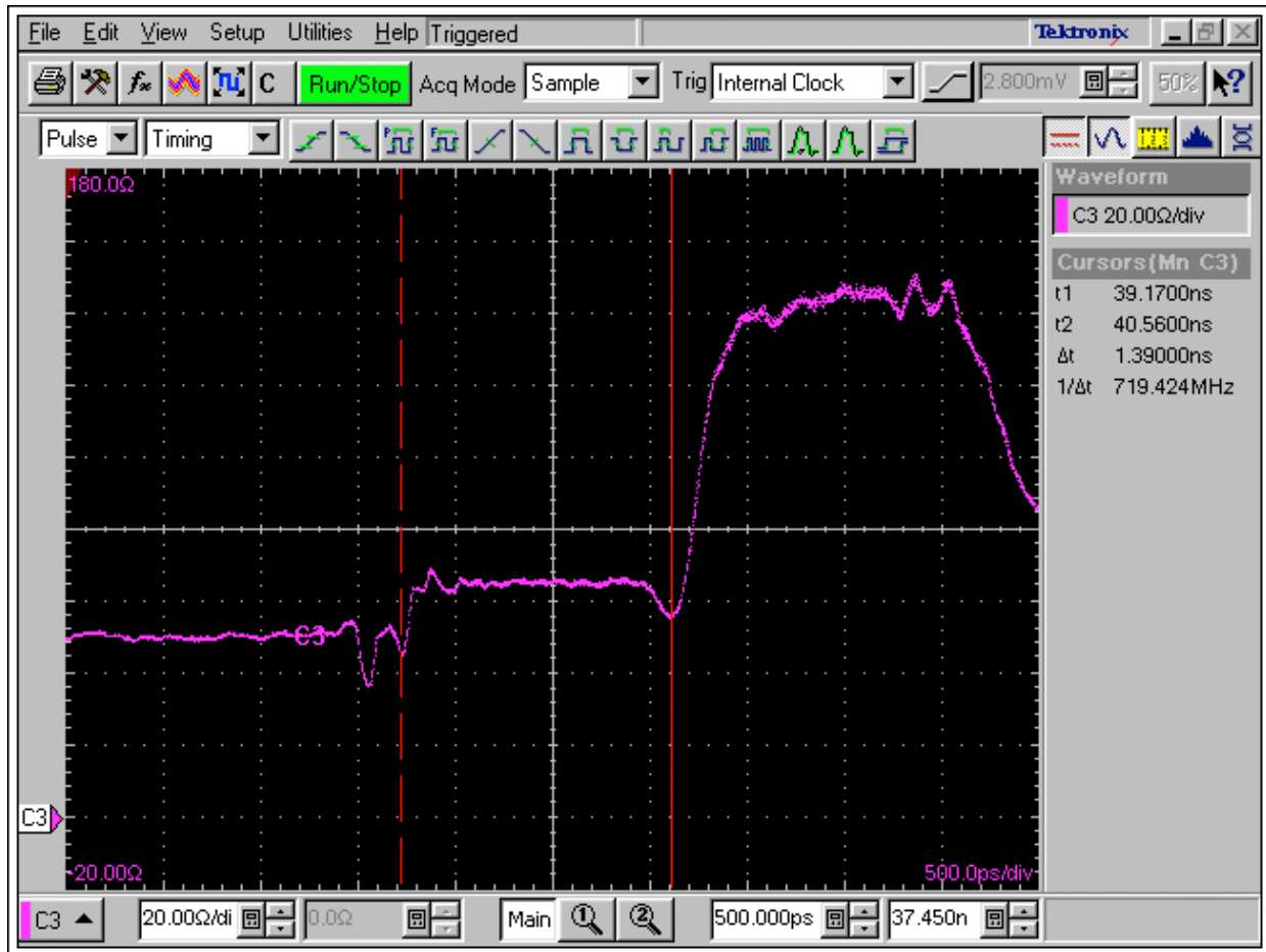
Figure 8. The same plot as Figure 7, but expanded and measuring delay.
