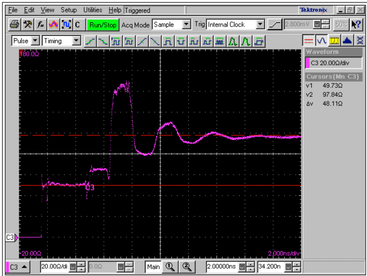
Figure 7. DATA1 PCB TDR impedance measurement.
