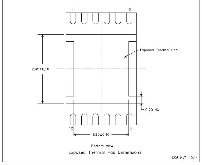
NOTE: All linear dimensions are in millimeters
