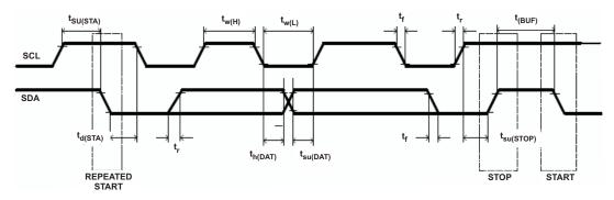
Figure 1. I<sup>2</sup>C-Compatible Interface Timing Diagrams
