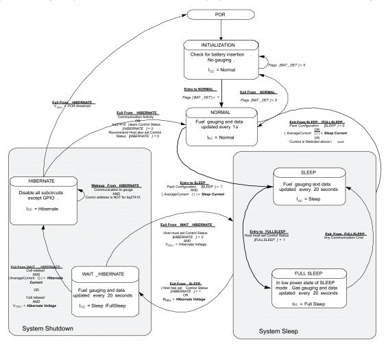
Figure 2. Power Mode Diagram
