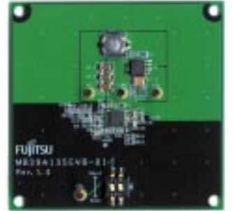
Photo 2 MB39A135 Evaluation Board (6.5cm×6.5cm)
