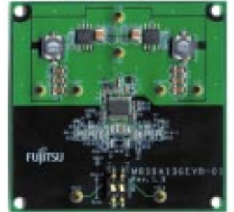
Photo 3 MB39A136 Evaluation Board (6.5cm×6.5cm)
